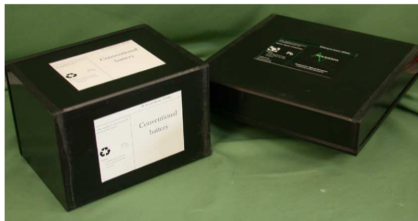
Fig. 8. Size comparison of conventional and Ebonex® bipolar 36 V lead-acid batteries.
